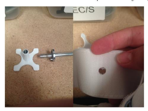
5. The metal stem will line up with the Black Plastic Hub and fit through the top hole. The side without the Velcro will be touching the black plastic hub. Screw the j-hook into the metal stem through the bottom of the hub. The metal stem will need to be pressed into the black plastic hub tightly so the j-hook reaches the metal stem.
